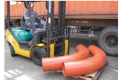
12" 3D 90° elbows ready for shipment
